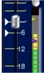
Figure 6.2: A fader with gain scale and meter
